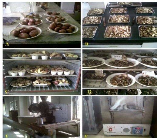
Figure 1: Sample Preparation from the tubers of selected potato germplasms. A) Washing of potato tubes, B) Cutting of potato tubers, C) Slice storage, D) Oven drying at 60 °C, E) Grinding of samples, F) Determination of total ash contents.
