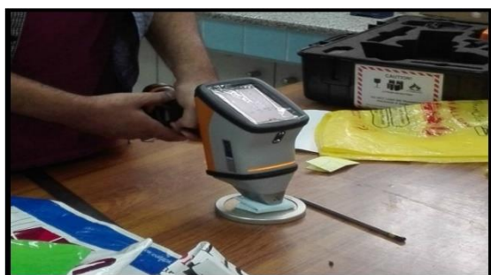
Figure 3: Analysis of plastic bag using HH-XRF.
